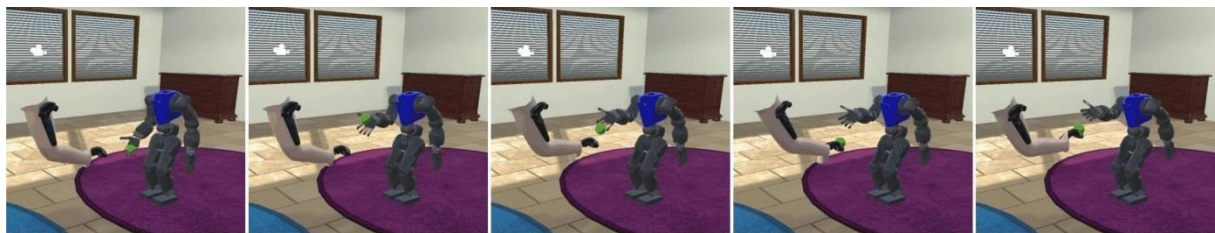
Fig. 2: Throwing sequence in VR generated by GAZEBO physics simulator of the robot.
