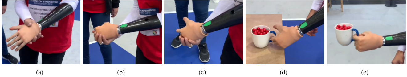
Fig. 3. The photo-sequence presents our strategy adopted to grasp a mug. The SoftHand Pro can change its shape according with the environmental constraints, and we exploited this feature to get a different closure shape.
