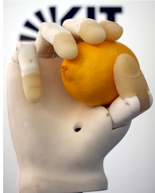
Fig. 1. The KIT Prosthetic Hand. The underactuation mechanism allows the fingers to adapt to the shape of the object.
