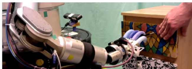
Fig. 1. A person holds a drawer shut while a robot tries to open it. Irrespective of such disturbances the robot can reliably open the drawer.
