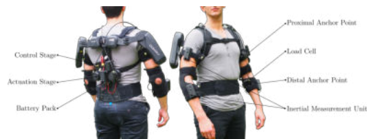
Fig. 1. Hybrid exoskeleton developed to assist elbow and shoulder joints.
