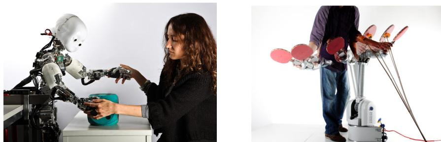
Kinesthetic Teaching: Guiding the robot through the motion Applicable to any type of robotic systems
