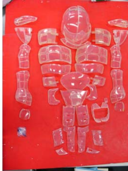
Covers by Rapid prototype(SLA)
