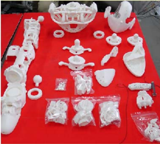
Bone by nylon Rapid prototype(SLS)
