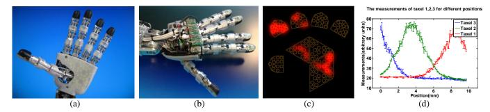
Fig. 1. (a) (b) Pictures of the hand. (c) An example of the visualization. (d) A graph indicating the crosstalk of the taxels.
